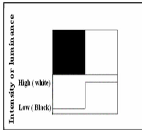
Figure 1: The Lighting method of schematically representing the edge. Increases to be bright from the right side
